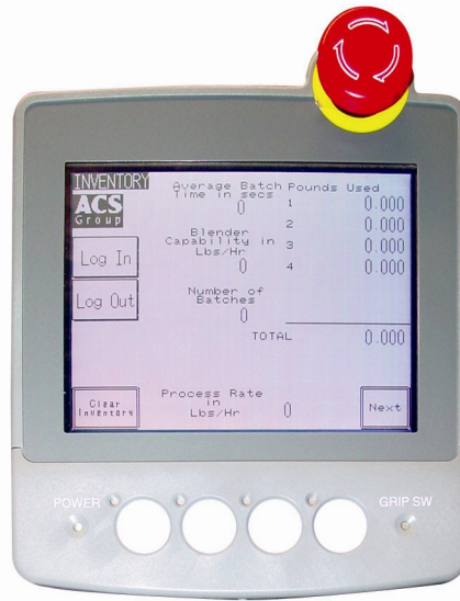
Figure 9: Typical Mitsubishi Controller Touch Screen Display
